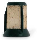
Prefilter of the E3T – blocked by rust
